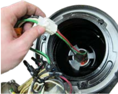
STEP 4: UNPLUG THE HID POWER LEADS FROM THE BALLAST ASSEMBLY
